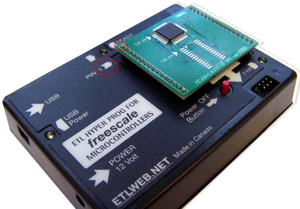
Figure 20 Proper adapter board insertion
