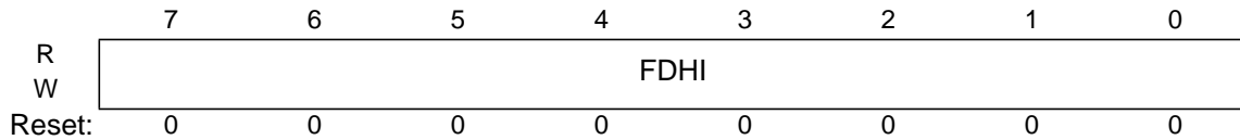
Figure 3-12 8-bit Flash Data High Register (FDATAHI)
